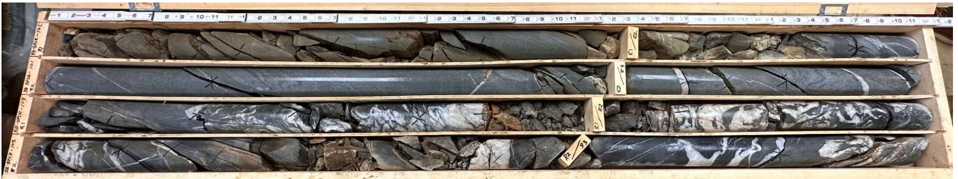
Top Row: BB-BPSR-101, Run No. R1: 8.5 ft (left) to 12.1 ft (middle-right), Run No. R2: 12.1 ft (middle-right) to 13.8 ft (right) Top Middle Row: BB-BPSR-101, Run No. R2: 13.8 ft (left) to 16.9 ft (middle-right), Run No. R3: 16.9 ft (middle-right) to 18.9 ft (right) Bottom Middle Row: BB-BPSR-103, Run No. R1: 7.0 ft (left) to 10.3 ft (middle-right), Run No. R2: 10.3 ft (middle-right) to 12.3 ft (right) Bottom Row: BB-BPSR-103, Run No. R2: 12.3 ft (left) to 14.9 ft (middle-right), Run No. R3: 14.9 ft (middle-right) to 17.0 ft (right)
